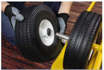
Slide the second wheel onto the axle, this time making sure the offset side faces inward. The offset sides of both tires should be facing each other.
