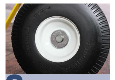
Slide the washer onto the axle.
